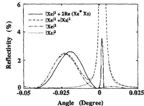
FIG. 2. Plot of various terms of Eq. (3) for a  $0.25\text{-}\mu\text{m}$   $\text{Al}_{0.25}\text{Ga}_{0.75}\text{As}/\text{GaAs}(001)$ . It shows that interference between the epilayer and substrate amplitudes is responsible for the epilayer peak shifting.
