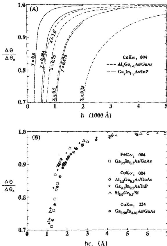
FIG. 3. (a) Plot of the separation between epilayer peak and substrate peak as a function of layer thickness. (b) Plot of the peak separation as a function of the product of thickness and perpendicular strain.
