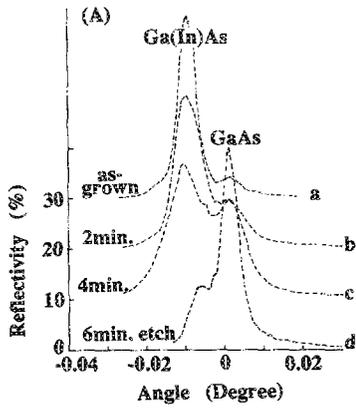
FIG. 1. (a) Experimental rocking curves of an indium-doped LPE GaAs layer on a GaAs substrate, taken after successive chemical etching. (b) Simulated rocking curves for different layer thicknesses.
