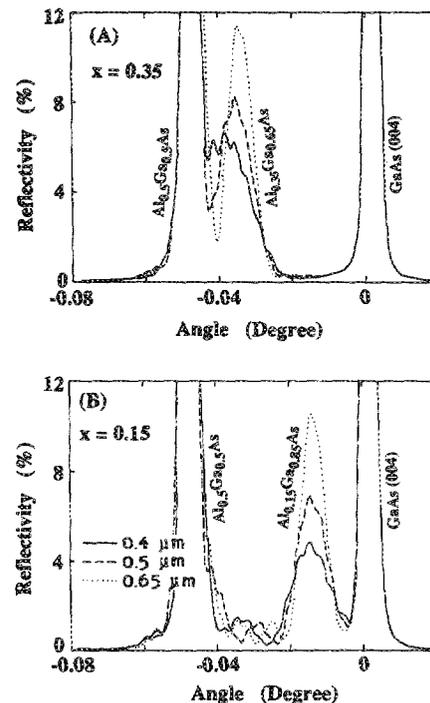
FIG. 4. Simulated rocking curves for 1.5- $\mu\text{m}$   $\text{Al}_{0.5}\text{Ga}_{0.5}\text{As}/\text{Al}_x\text{Ga}_{1-x}\text{As}/1.5\text{-}\mu\text{m}$   $\text{Al}_{0.5}\text{Ga}_{0.5}\text{As}/\text{GaAs}$ (001) for  $x =$  (a) 0.35 and (b) 0.15 at varying thickness of the  $\text{Al}_x\text{Ga}_{1-x}\text{As}$  layer. The thicknesses are the same in (a) and (b).
